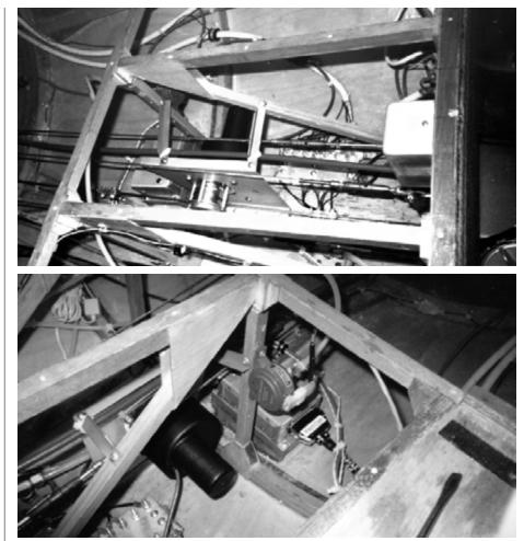
Also, the pedestal below the panel must be moved aft by the same amount and the center console trimmed to fit. (By the way, this relocation of the panel relieves some of the strain on the three connector plugs at the back of the panel and provides a little more room to remove individual instruments when necessary.)
