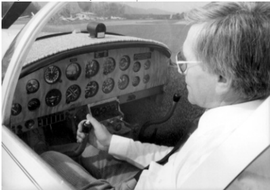
Below: Herbert Müller's instrument panel is made in two pieces, with the top half removable.
