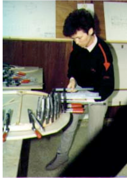
Above: Mrs. Bjoern Eriksen working on a fuselage frame. This photo was taken in 1983 and this Falco project in Norway is now taking shape rapidly.
