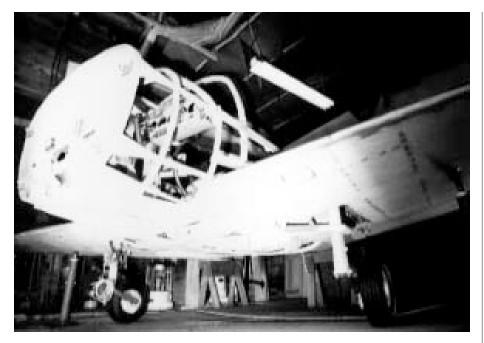
is the airplane's Jesus joint—wing centersection clasping the cockpit area in, one hopes, a permanent embrace.
