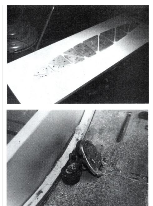
Top: A wing rib jig takes shape. The Baltic birch plywood blocks are positioned with dowel pins. Bottom: Stephen Friend's method of machining the fuselage frames to thickness using roller skate wheels to hold the frame against a fence.
