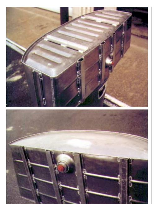
The aft tank passed the slosh and vibration test with these four hat-section braces installed on the bottom. The front fuel tank in this configuration survived 9 hours of the test and then failed. It will required 8 braces on the bottom.
