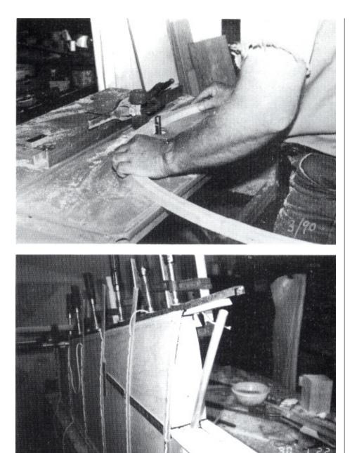
Top: Stephen Friend thicknessing the fuselage rings on the inside. The roller skate wheel determines the thickness. Bottom: Stephen clamps the leading edge skin in place with a steel channel.
