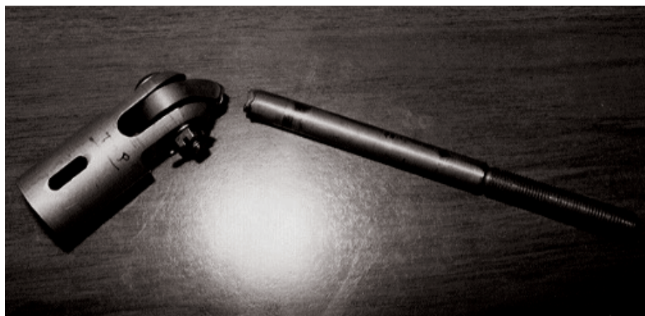
Below: Jonas Dovydenas's nose gear retraction pieces that failed.
