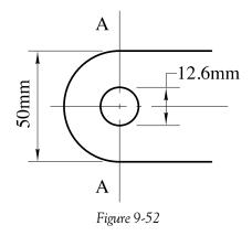
The diametric projection of the pin supporting surface is:
