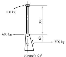
With a simple calculation, we obtain the effort on the stick pin of 600 kg and on the limit stops of 500 kg. A bolt with a 6 mm diameter is enough for the stick pin. The resisting surface is, in fact:
