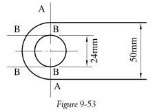
Let's verify again, based on the 7mm thickness of the plate, the tensile eye in section A-A without considering the washer contribution. The verification in section *B-B* is superfluous, since in this case the shear resisting area is greater than the tension resisting area.
