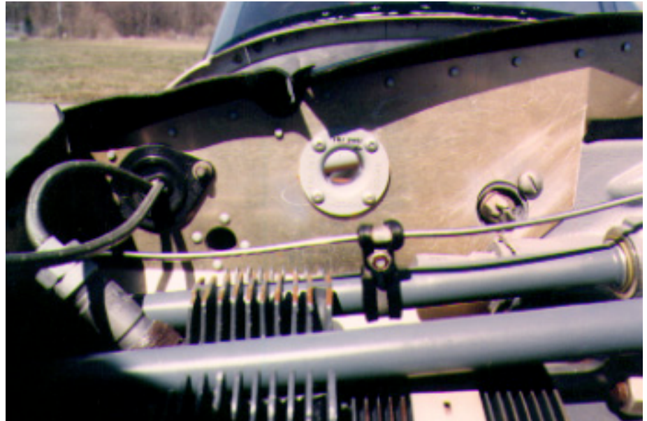
The plastic flange is installed on the right baffle.
