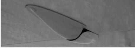
Larry Black put a radius on the rudder fairing, removed an external bent-wire com antenna, installed flush screws on the cowling and these trailing fairings on his ailerons and flaps. All these gave him a speed increase of about 12 kts, which sounds far-fetched but he can now outrun John Harns and Dave McMurray, who used to be faster than him. In formation, Larry pulled 2400 19" to John and Dave's 2400 23".
