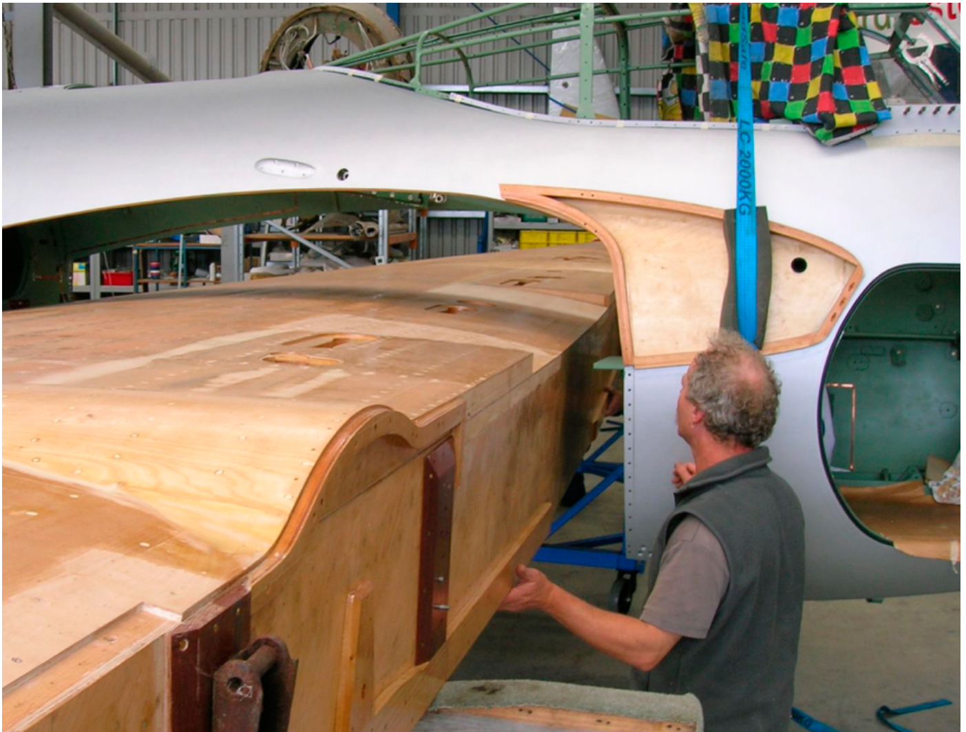
The spruce wing spars span 50 feet tip to tip.
