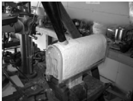
Vacuum cleaner hose attached to the plastic. Note the gray glaziers tape sealing the hose. The glaziers tape around the perimeter of the plug isn't necessary if a plastic bag is used.
