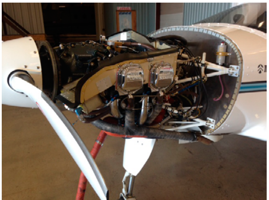
Top: N1443D High Performance engine (193 hp) – Built by Mena Aircraft Engines Middle: GT V29 composite blade. Above: N1443D high performance engine and GT Composite propeller.
