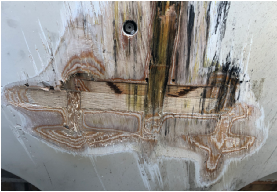
The main wing spar sits on top of the bottom center longeron, so it is not damaged at all, but this does show that an external wear strip on top of the skin would help a lot.
