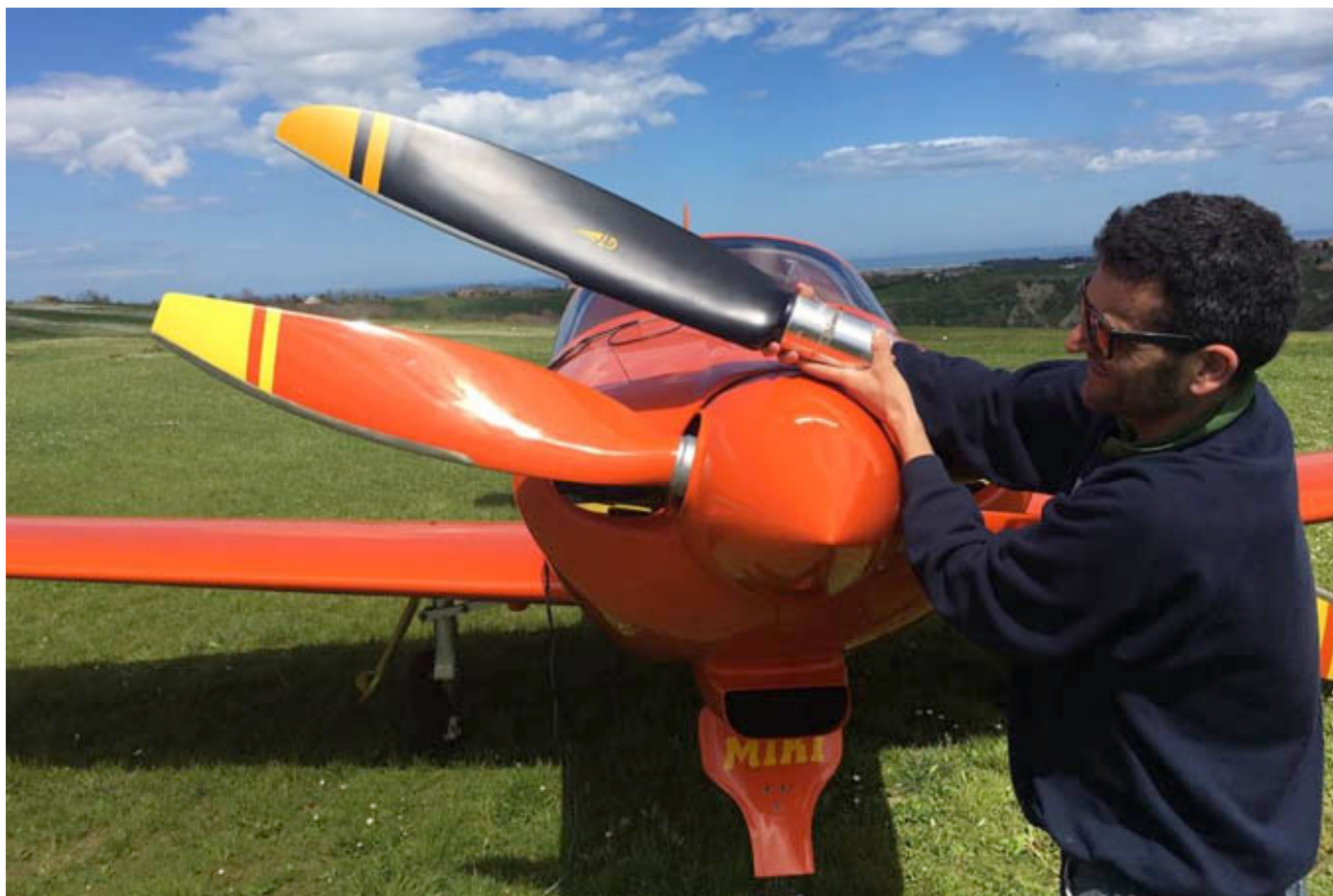
Alex Tonini showing the new GT2V46 blade design based on the original Rotol Spitfire propeller.
