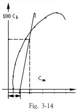
The value of the coefficient of moment in relation to zero lift,  $C_L$  = 0, is of particular importance in determining the airfoil's stability. This intersection on the horizontal axis is called  $C_{\rm m0}$ . The position of the center of pressure may be determined graphically in the polar chart by looking at the moment curve.
