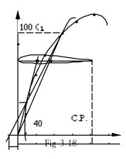
Case C. Let's now consider the third condition. For zero lift,  $C_{m0}$  is negative. The effect of the center of pressure is therefore opposite the one noticed in Case A. For an increase in incidence, the C.P. will move toward the trailing edge, and forward when the angle of incidence is reduced. In these conditions, the airfoil is stable.
