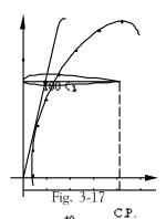
Case B. In this case,  $C_L = 0$ ,  $C_{m0} = 0$ , and the curve goes through the origin. From the chart we note that for any variation the position of C.P. does not move, and it coincides with the focus of the airfoil. An airfoil with this characteristic is said to have neutral stability.
