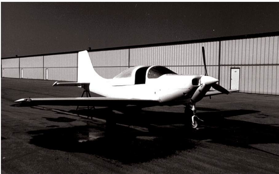
Above center: Willard Hofler's Falco lacks only the cowling, prop and interior. Bottom: Butch Harbold's Sequoia 300 nears completion but is very seriously tail-heavy and will require a ten-inch movement of the engine to get it in balance.
