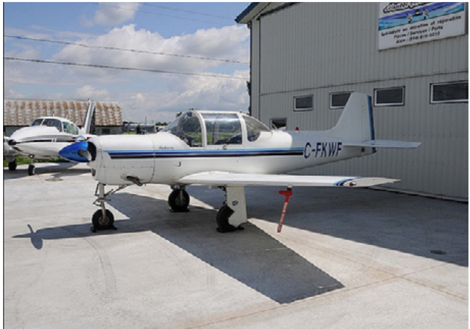
Dwight Lapeare first flew his Falco in April 1997. Now with a Lycoming O-320-A1A and constant-speed prop, Dwight says it gets him out of a 2200' grass strip with a full load. "A dream to fly" he says. We've asked Dwight to give us a full report in a future builder letter.
