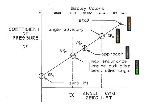
Angle-of-attack as a function of the pressure coefficient and corresponding LED indications
