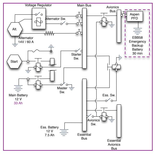
Schematic Electrical Diagram of I-DIET
