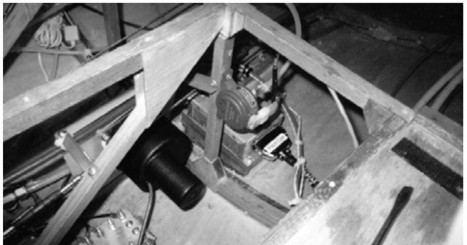
Also, the pedestal below the panel must be moved aft by the same amount and the center console trimmed to fit. (By the way, this relocation of the panel relieves some of the strain on the three connector plugs at the back of the panel and provides a little more room to remove individual instruments when necessary.)
