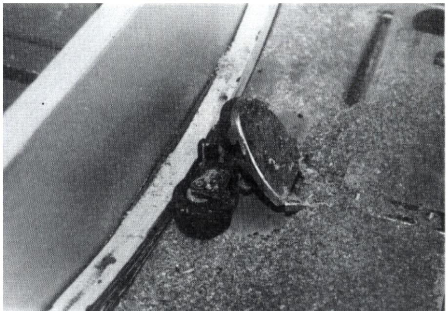
**Top:** A wing rib jig takes shape. The Baltic birch plywood blocks are positioned with dowel pins. **Bottom:** Stephen Friend's method of machining the fuselage frames to thickness using roller skate wheels to hold the frame against a fence.
