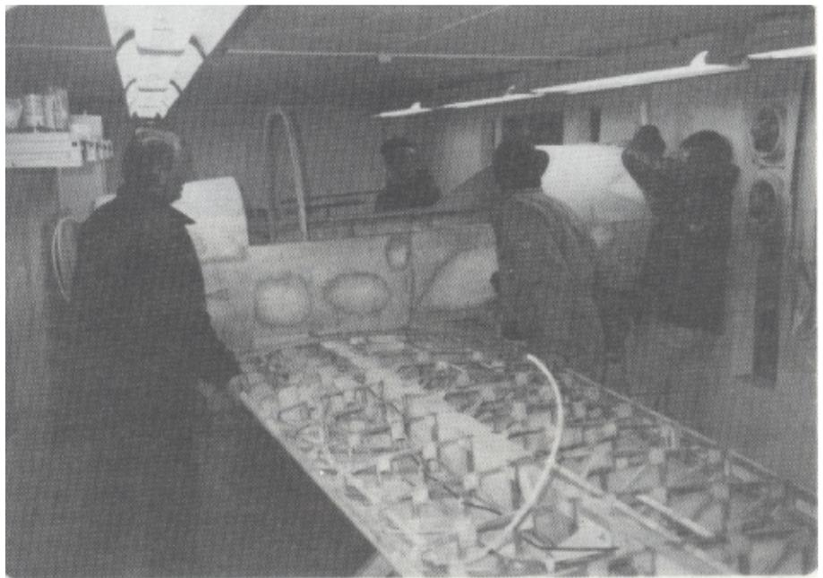
canopy, engine mount, engine, nose gear, and cowling were all completed before the wing was begun. The tail section was cut off and prepared for painting, as well as a short section of the fuselage centersection to ensure a perfect fit after final assembly.
