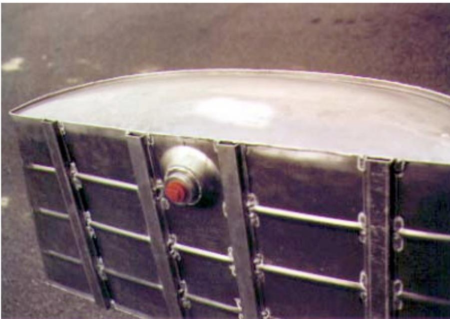
***The aft tank passed the slosh and vibration test with these four hat-section braces installed on the bottom. The front fuel tank in this configuration survived 9 hours of the test and then failed. It will required 8 braces on the bottom.***
