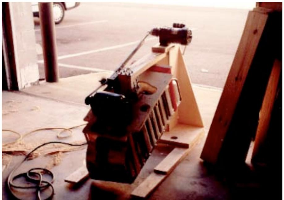
*The slosh and vibration test rig with the forward fuel tank. A motor over the tank swings an eccentric weight on a shaft to provide the vibration, while a gear-motor with an eccentric arm connected to a pushrod provides the sloshing.*
