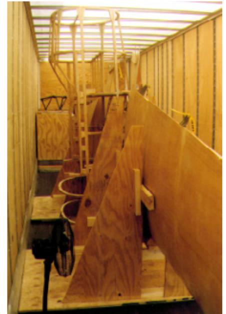
use of the trailer. We loaded the engine, crates, boxes and propeller in the front of the trailer, and partitioned that section off. The two main structures were loaded in the center. Last to be loaded was the plywood and jigs used for setup.
