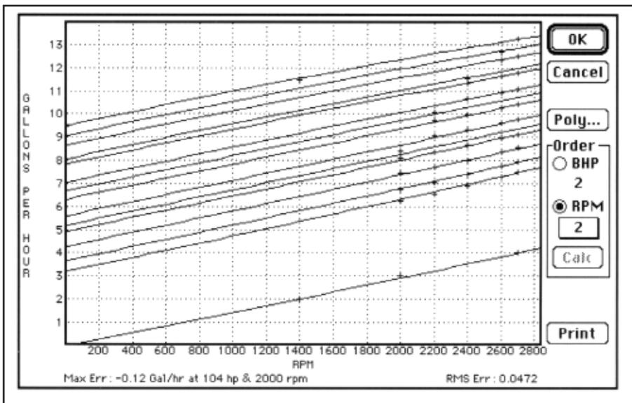
**Top: Curve-fitting the fuel flow of the engine. This is a three-dimensional curve—shown here is brake horsepower vs gallons per hour. Above: Here’s the same curve plotted with revolutions per minute vs gallons per hour.**
