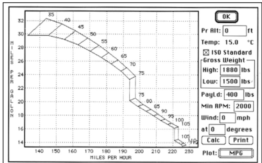
Top: The real fun begins when you use the airspeed calculator, which shows curves for power required and power available. The speed in level flight is where the two curves cross at the right. Maximum excess horsepower translates to the best climb speed and rate. Above: Here's the way the miles-per-gallon chart looks on the screen.
