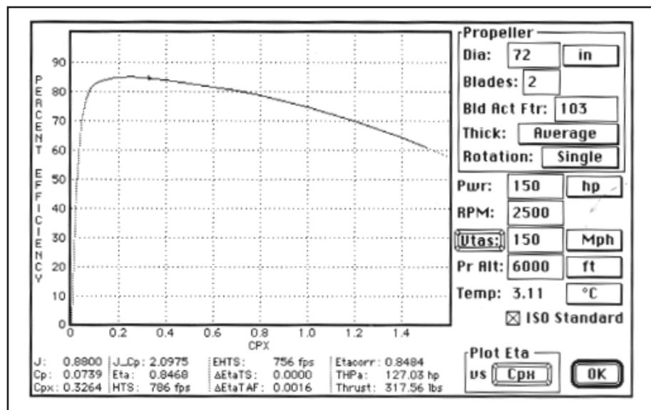
**Top:** The propeller efficiency calculator showing the traditional view of efficiency (Eta) vs  $J/Cp^{1/3}$ —which is the propeller advance ratio divided by the cube root of the coefficient of power. **Above:** Another view of the same thing, but looking 'side-ways' through the three dimensional curve. Here you see Eta vs  $Cpx$ —which is the adjusted coefficient of power.
