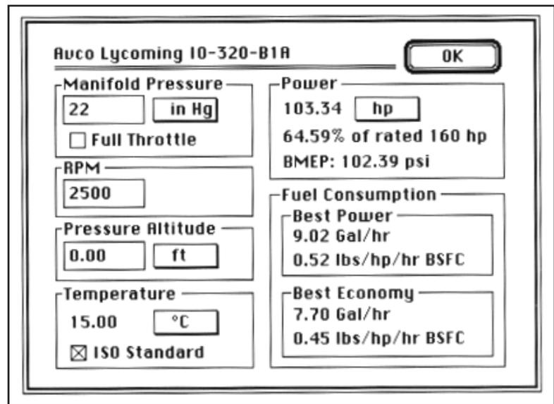
*Top: Curve-fitting the maximum engine horsepower vs rpm. You click on the icons in the lower right to zoom in and out. Above: Once the engine is modeled, you can use the engine power calculator.*
