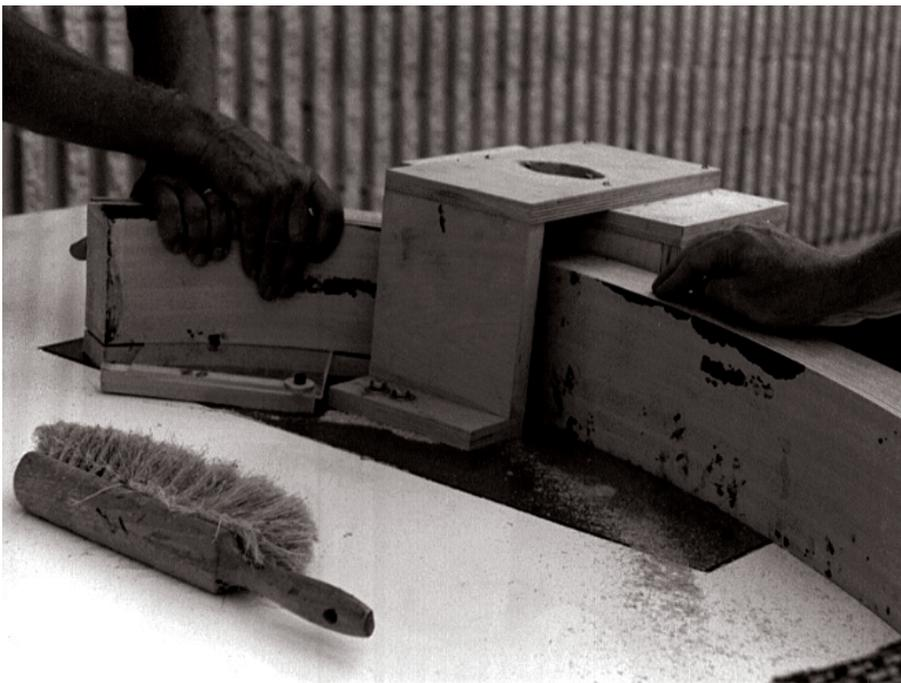
*Top: Our modified shaper with the tall spindle and saw blade in place.
