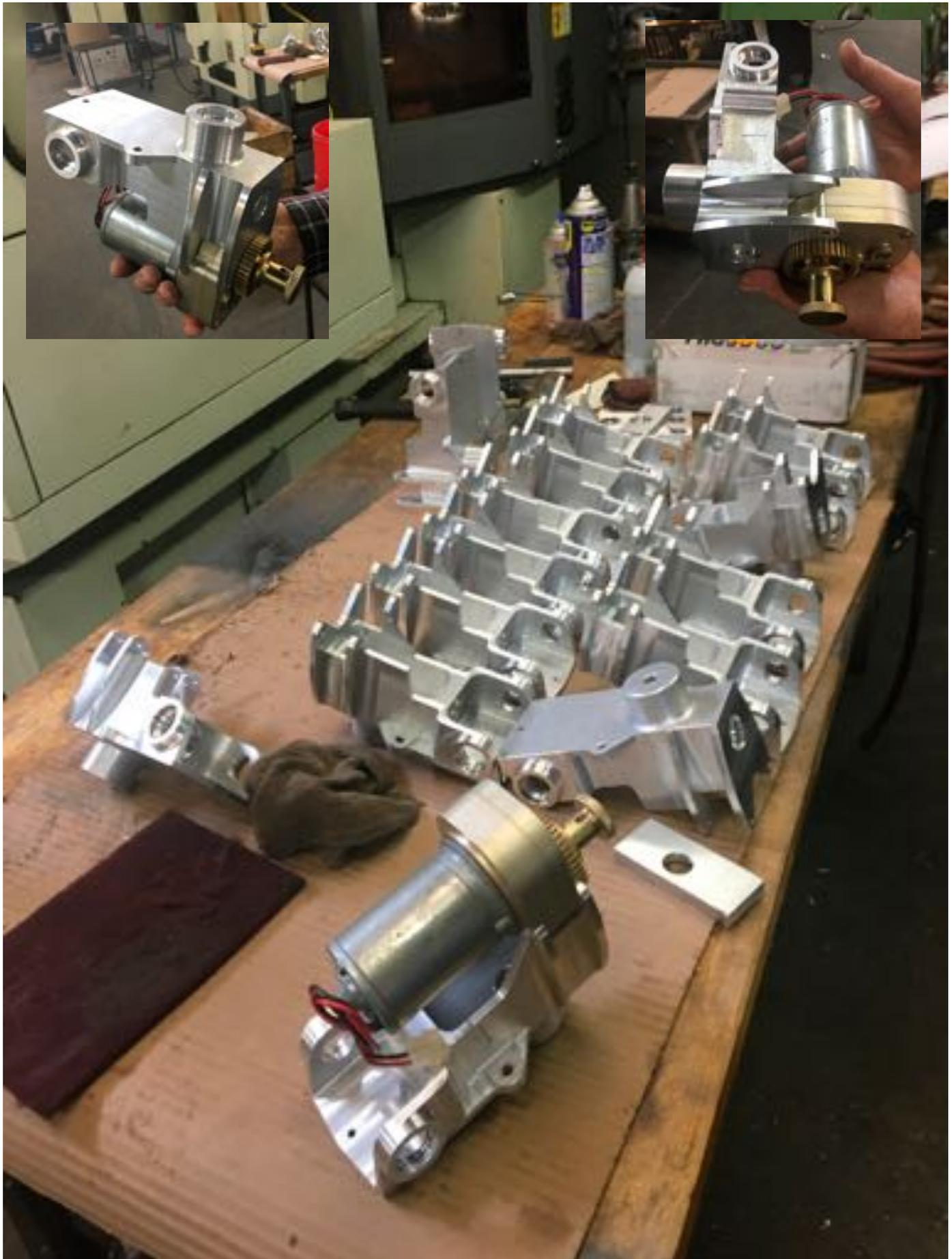
*Here's the P/N 520 Gearbox, now being machined from a solid forged block of 6061T6. There is a limited supply, first come first serve. Get your orders in with Gunder.*
