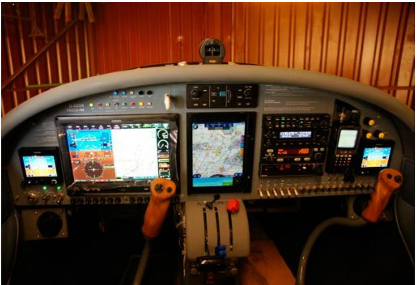
the decision was made to substitute more modern LED indicator lights. This led to another change, in that the original indicator lights couldn't be dimmed, whereas the new ones can — by way of a pulse width modulator and mosfet installed on a common ground circuit. One twist of a knob and all indicator lamps dim together.
