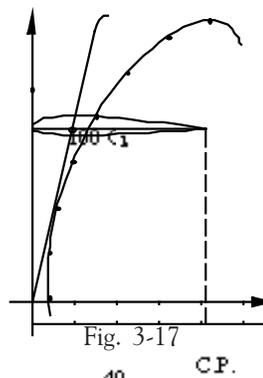
Case B. In this case,  $C_L = 0$ ,  $C_{m0} = 0$ , and the curve goes through the origin. From the chart we note that for any variation the position of C.P. does not move, and it coincides with the focus of the airfoil. An airfoil with this characteristic is said to have neutral stability.
