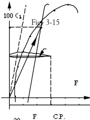
For a given value of  $C_L$ , a horizontal line is drawn with its origin on the vertical axis and its length equal to the value of  $C_m$ , i.e.  $100 C_L = 30$ ,  $100 C_m = 30$ . This line is called the reference chord.
