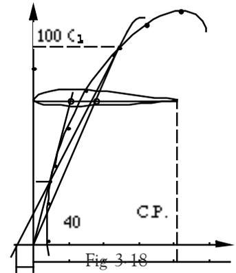
Case C. Let's now consider the third condition. For zero lift,  $C_{m0}$  is negative. The effect of the center of pressure is therefore opposite the one noticed in Case A. For an increase in incidence, the C.P. will move toward the trailing edge, and forward when the angle of incidence is reduced. In these conditions, the airfoil is stable.
