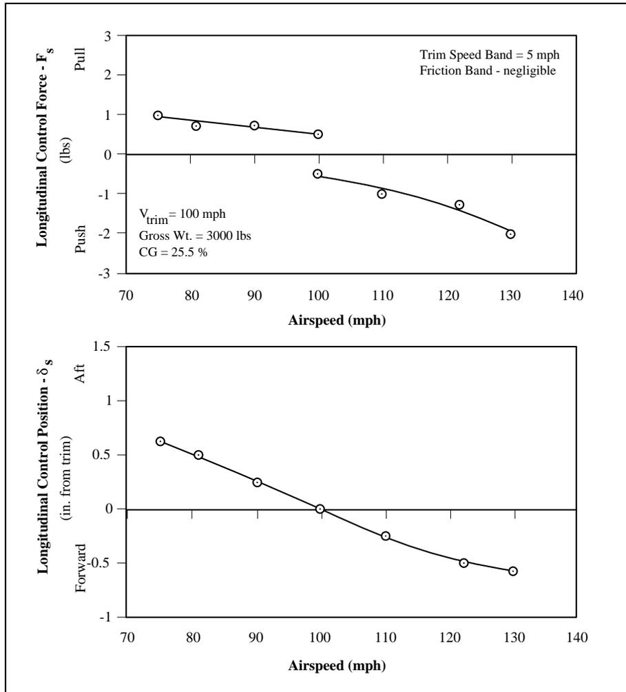
**Figure 5. Sequoia 300 Longitudinal Stability Characteristics, Configuration PA—Aft CG**
