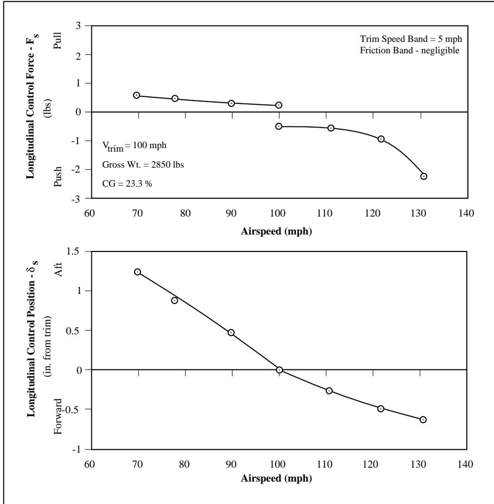
**Figure 4. Sequoia 300 Longitudinal Stability Characteristics, Configuration PA—Mid CG**
