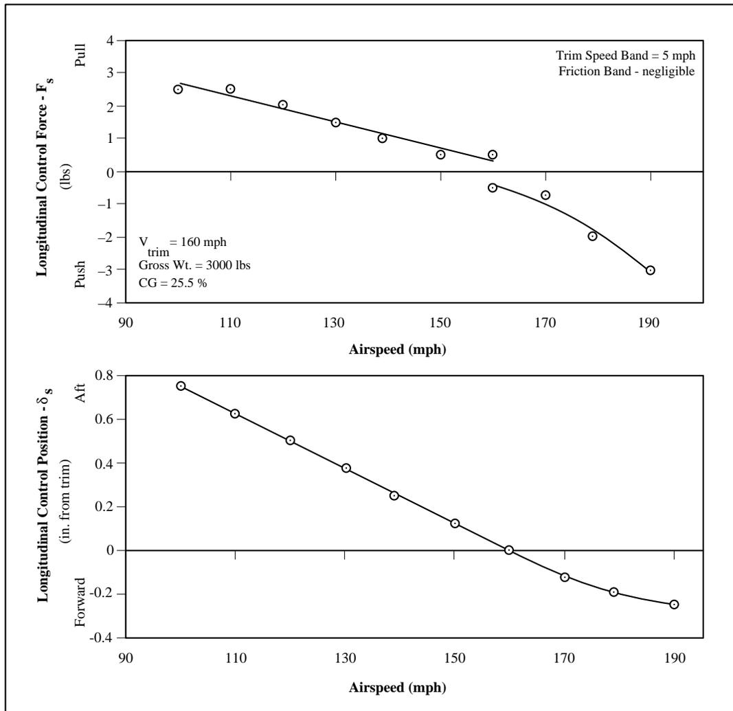
**Figure 3. Sequoia 300 Static Longitudinal Stability Characteristics, Configuration CR—Aft CG**
