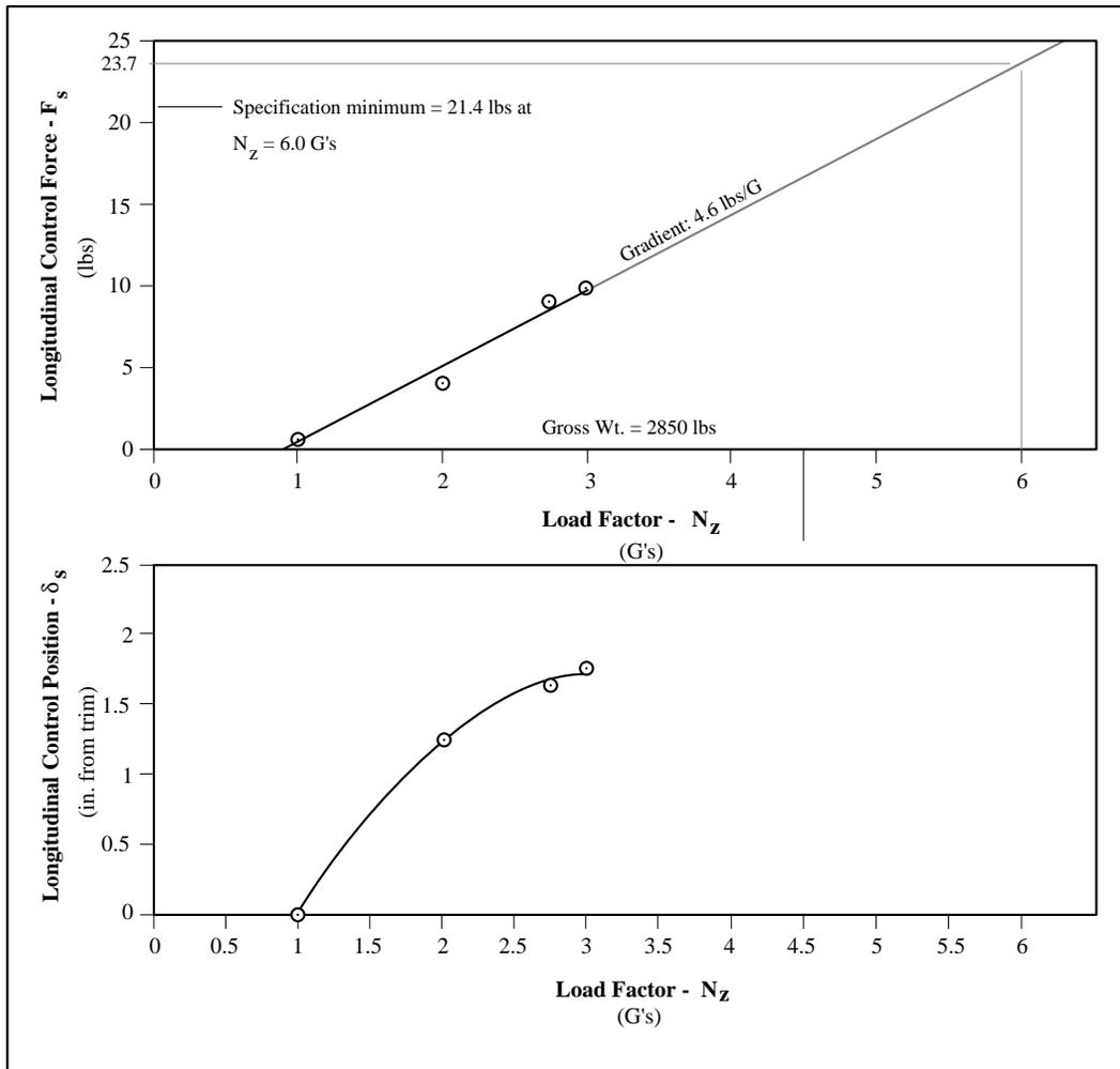
**Figure 7. Sequoia 300 Maneuvering Longitudinal Stability Characteristics Configuration CR**
