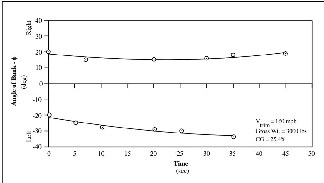
**Figure 11. Sequoia 300 Spiral Mode Configuration CR—Aft CG**
