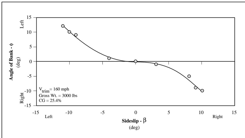
**Figure 10. Sequoia 300 Sidforce Characteristics Configuration CR—Aft CG**
