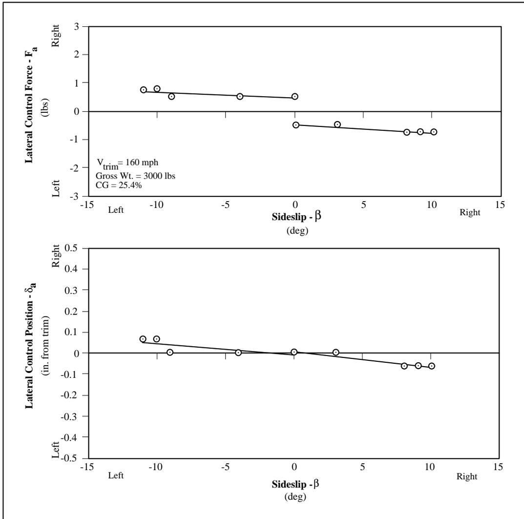
**Figure 9. Sequoia 300 Dihedral Effect Characteristics Configuration CR—Aft CG**
