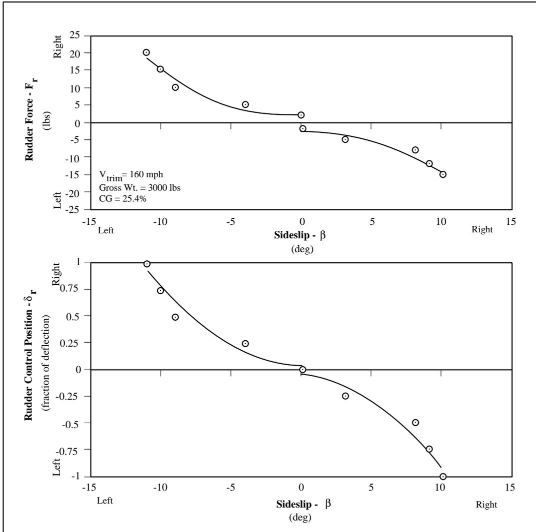
**Figure 8. Sequoia 300 Directional Stability Configuration CR—Aft CG**
