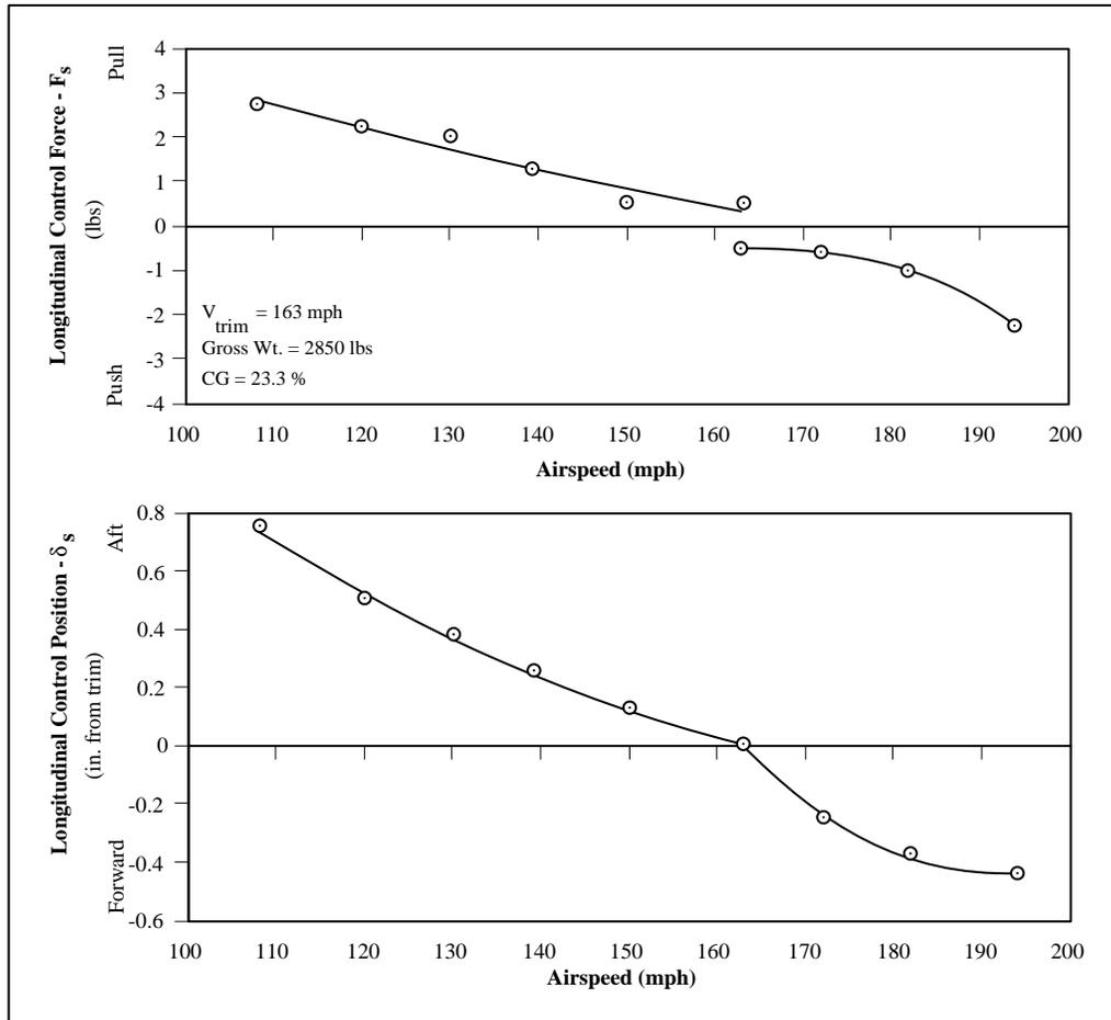
**Figure 2. Sequoia 300 Static Longitudinal Stability Characteristics, Configuration CR—Mid CG**
