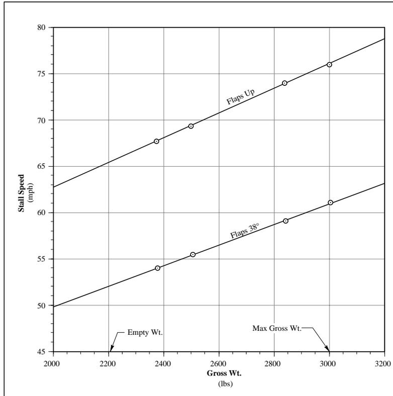
**Figure 12. Sequoia 300 Stall Speeds Configurations CR and PA**
